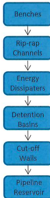
FIGURE 6-2 Surface Drainage Flow Diagram
